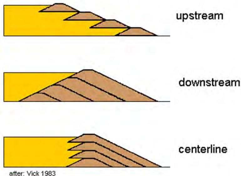
Downstream construction is the safest type of construction from a seismic standpoint, but is also the most expensive option.
